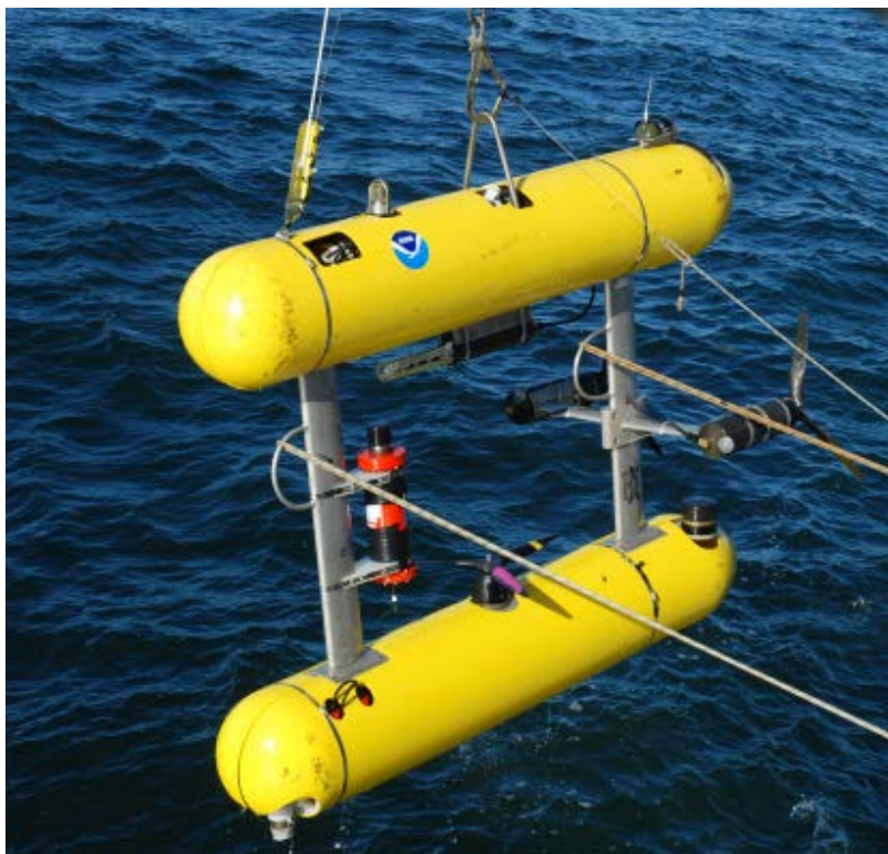
The AUV Lucille coming on board the research vessel. With negative buoyancy in the lower hull, and positive buoyancy in the upper hull, Lucille is able to remain stable in the unpredictable pitch and roll of the ocean while it follows the terrain of the bottom. Image courtesy of San Andreas Fault 2010 Expedition, NOAA-OER. http://oceanexplorer.noaa.gov/explorations/10sanandreas/background/auv/media/recovery1.html
